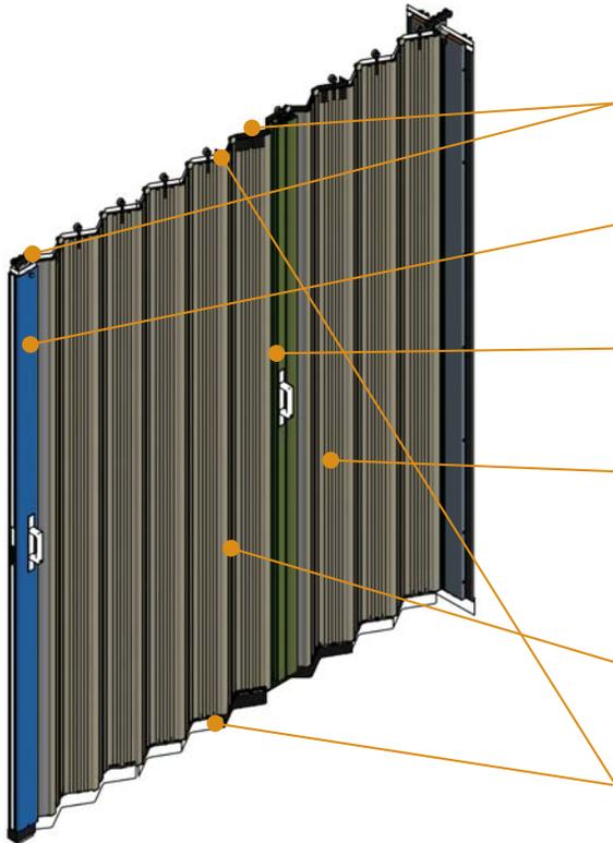
**TRACK** - Heavy-duty extruded aluminum or steel supports and retain the roller assemblies.
